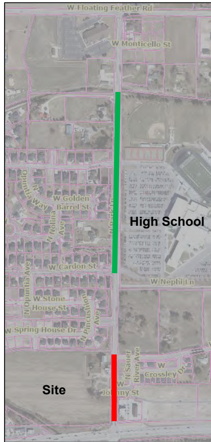
Park Lane - Existing center turn lane extents are in green, and Skyview Subdivision will be required to construct a center turn lane and extend the southbound left-turn lane at the intersection of SH-44/Park Lane.
