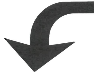
A=16 SF LEFT/RIGHT TURN ARROW (For the right turn arrow, use the mirror image.)
