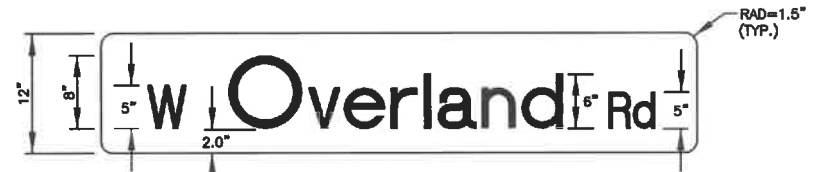
STREET NAME SIGN DETAIL FOR: MULTI-LANE PUBLIC STREETS, SPEED LIMIT 45 MPH OR GREATER
