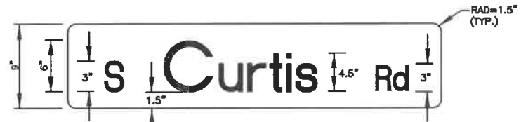
STREET NAME SIGN DETAIL FOR: MULTI-LANE PUBLIC STREETS, SPEED LIMIT LESS THAN 45 MPH TWO-LANE STREETS (ANY SPEED LIMIT) PRIVATE STREETS
