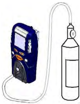
Figure 4.1 Bump Test / Gas calibration set up
